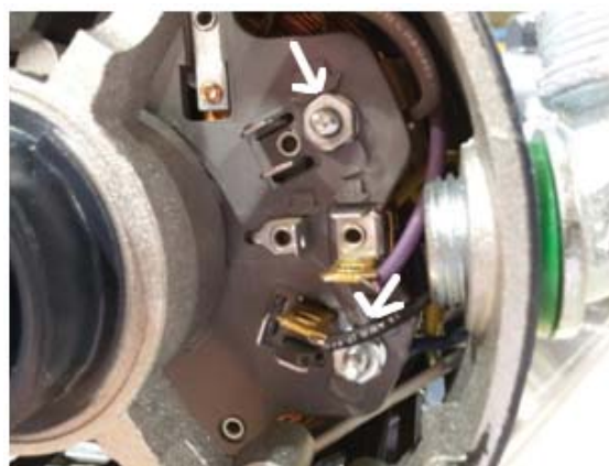
Line connection spades for L1, Neu (arrow 1 & 2)
