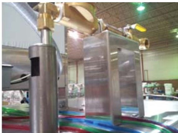
Showing hot water inlet, solenoid, and air gap
