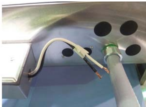
Showing power connection box for 120v wiring
