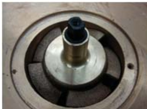
Drain axial propeller, o-ring on shaft
