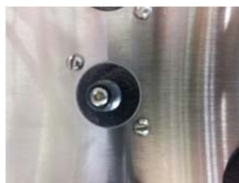
Chemical alarm barb adjusting screw *
