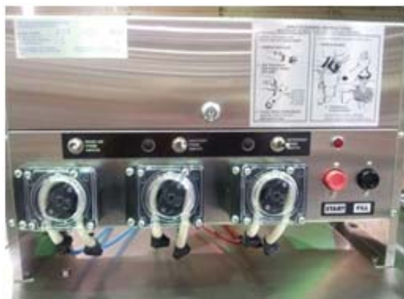
Showing deter, rinse, sanitizer pumps
