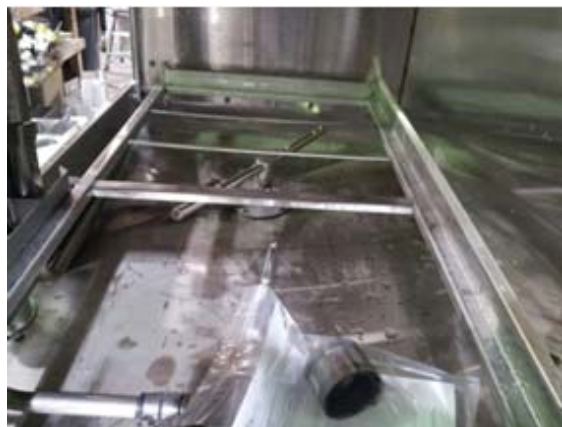
Corner-double tray track assembly (left-front)
