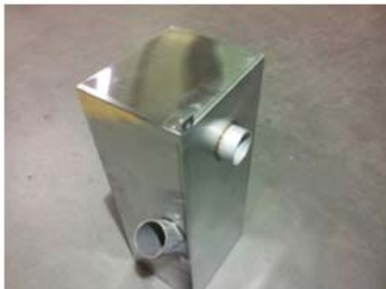
Showing 3DS bottom & side exit scrap box
