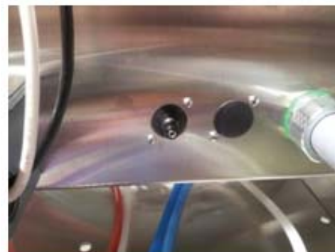
Chemical alarm barb adjusting screw *
