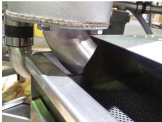
Correct alignment for sump to box
