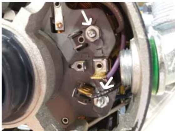
1.5 HP Motor, arrow 1 arrow 2 point to L1 & Neutral connect points
