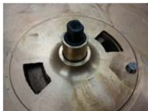
Drain inlet plate, w/alignment screw
