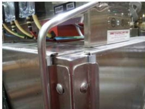
Showing correct arm alignment
