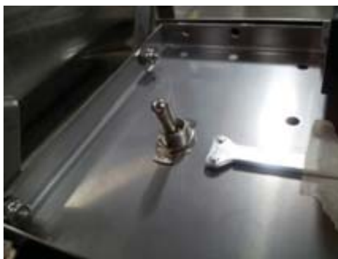
De-lime switch in control box
