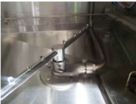
Spray arm, base w/thumb screws
