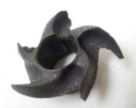
Impeller damaged from high acid solution
