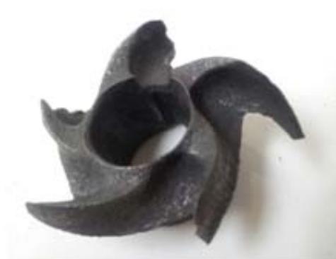
Impeller damaged from high acid solution
