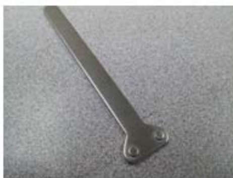
Cam timer adjustment tool
