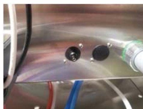
Chemical alarm barb adjusting screw
