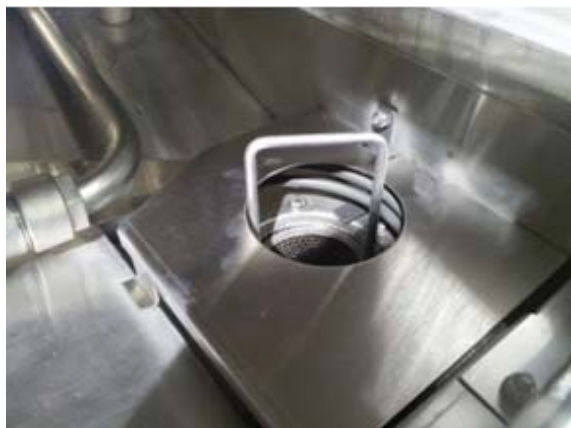
Sustainer heater cover and pump filter system
