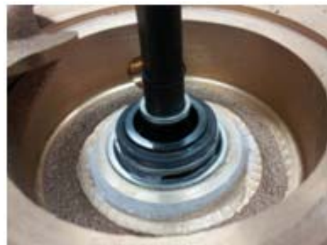
Graphite seal pressed into pump base
