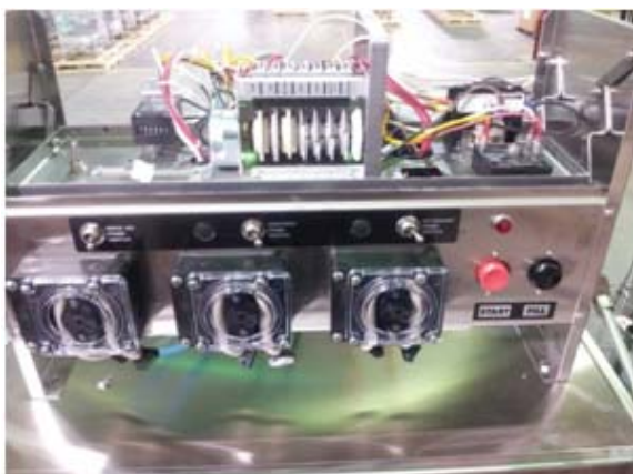
Showing control box, chemical pumps, prime switches
