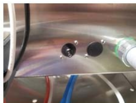
Chemical alarm barb adjusting screw *
