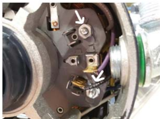
Showing connection points in 1.5 HP, 120v motor black & white wires attach to spades left of the two nuts
