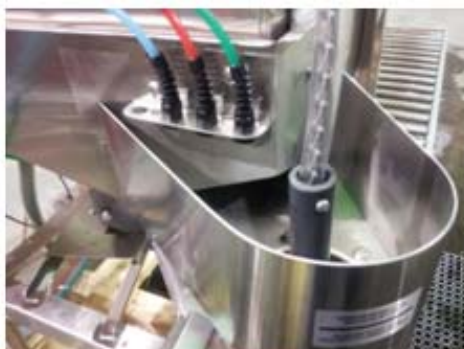
Showing 3DS sump, drain ball, water-level decal, chemical tubes
