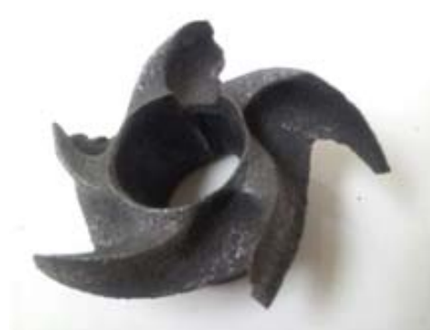
Impeller damaged from high acid solution
