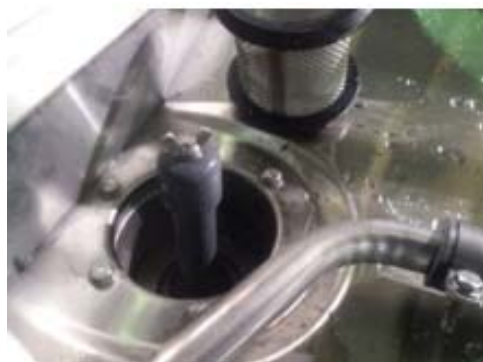
Showing sump, drain ball, pump filter
