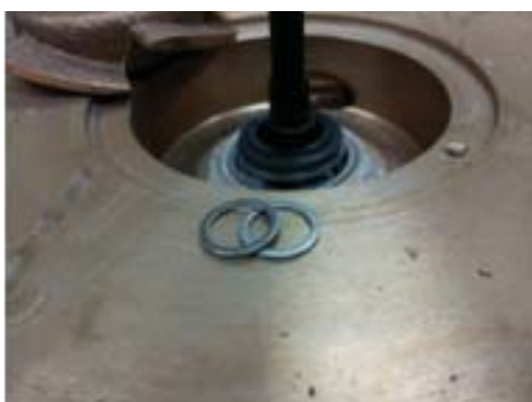
2 Spacer washers under propeller APPENDIX
