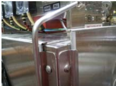
Showing misaligned arms on corner
