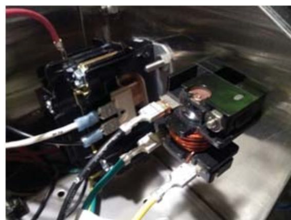
Wash motor contactor and motor relay
