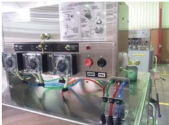
Showing deter, rinse, sanitizer external pumps
