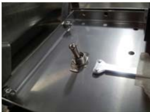
De-lime switch in control box
