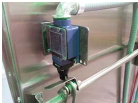
5-AGS Door cut-off switch and lever arm
