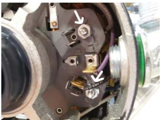
Showing connection points in 1.5 HP, 120v motor black & white wires attach to spades left of two nuts
