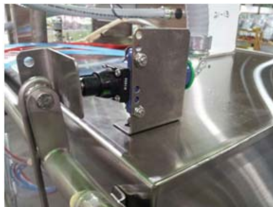
5-CD Door cut-off switch and lever arm
