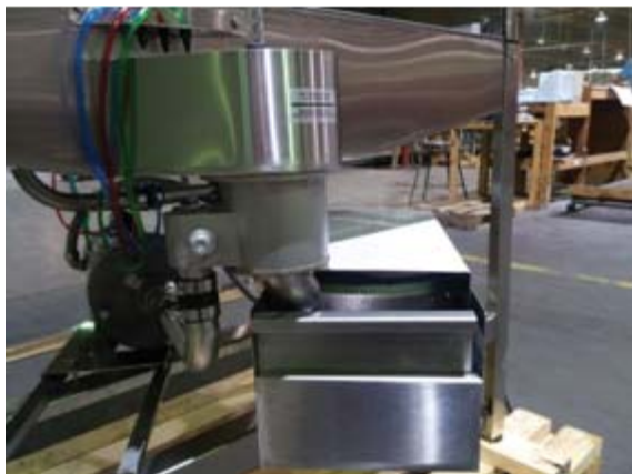
Showing scrap box as installed on 5-CD R-F
