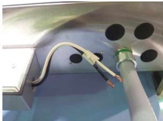
Showing power connection box for 120v wiring
