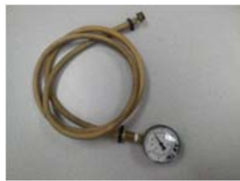
Spray arm pressure tester # 088-1048
