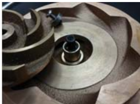
Impeller removed from housing
