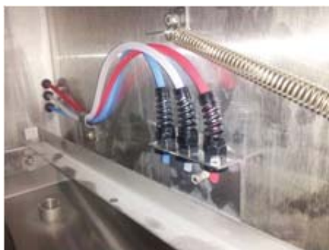
Showing chemical lines above sump
