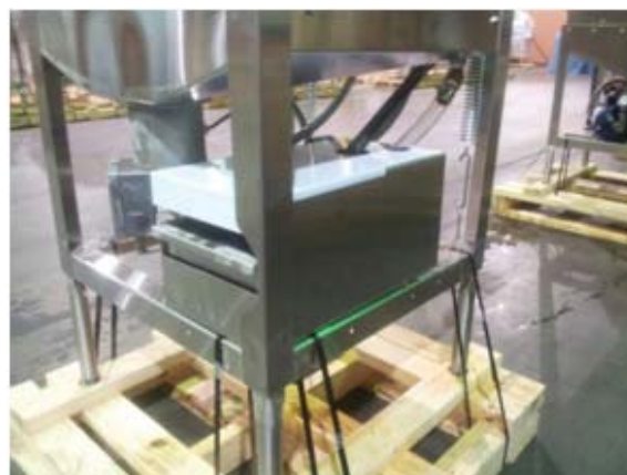
L-3DW-S scrap box in-frame mounting
