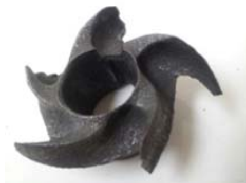
Impeller damaged from high acid solution
