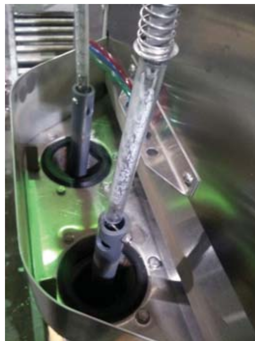
Dual drain balls, sumps, and pump filters
