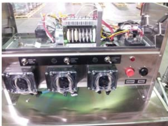
Showing control box, chemical pumps, prime switches
