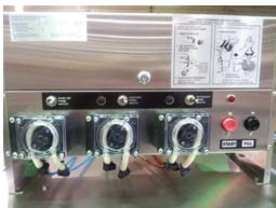
Showing 3DS detergent, rinse, sanitizer external pumps
