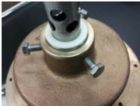
Diffuser w/spray arm pivot
