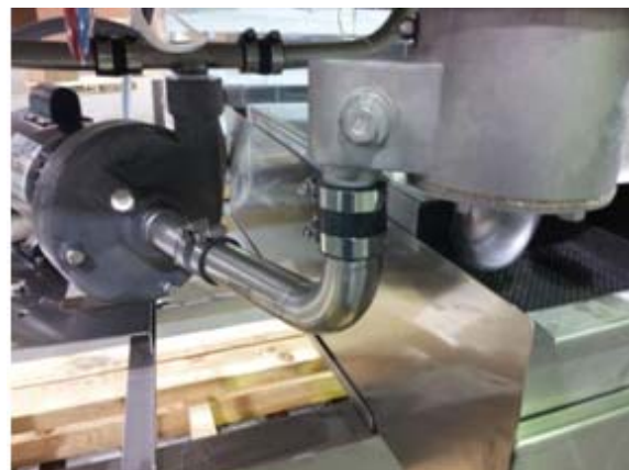
Single Pump, intake and discharge manifolds
