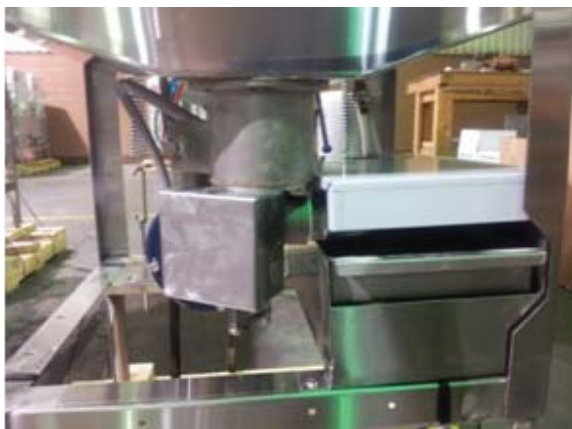
Showing L-3DW-S internal sump and scrap box
