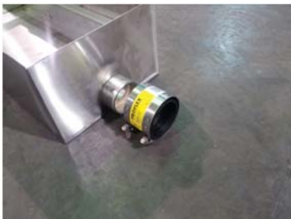
Showing the scrap box drain hub connection
