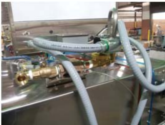
Showing 1/2" female pipe inlet, ball valve, y-line filter, water solenoid,
