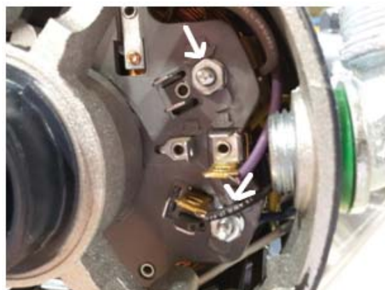
Line connection spades for L1, Neu (arrow 1 & 2)
