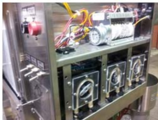
AFB prime switches and internal chemical pumps
